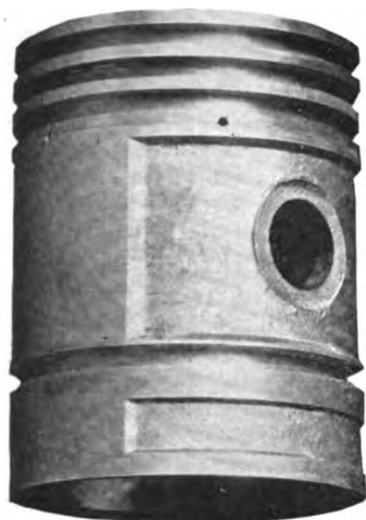
Northway adaptation of the hour-glass type of aluminum alloy piston which fulfills the requirements for this type of casting
